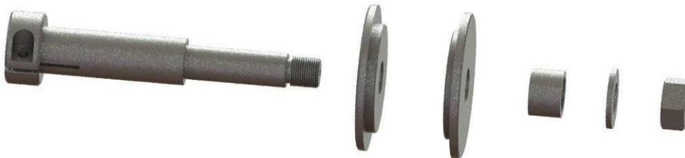
Cylindrical wheel arbor Spindle Dia: Ø16 mm Washer: Ø 68 mm (2x) Brush width: 20-40 mm PART NO: 7324-SPB_84S_G130
